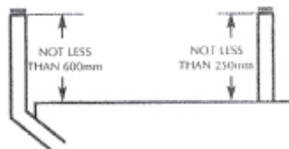
FLAT ROOF WITH NO PARAPET
