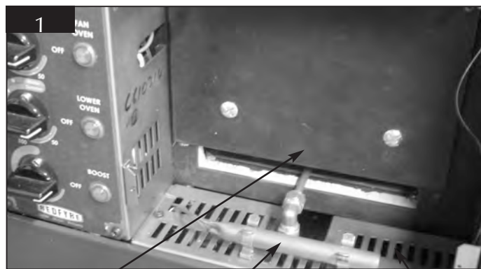
Burner door KBB fire valve phial Lower cover plate
