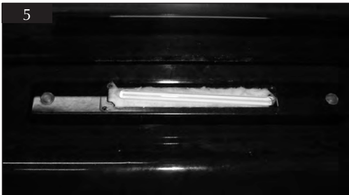
4.7 Refit temperature scale, ensuring thermometer sits correctly.
