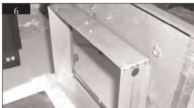
1.6 Locate top oven transfer box into aperture in front panel. Continue following these On-Site Assembly Instructions from Top Oven (2.1)
