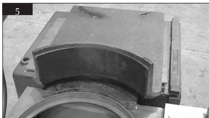
1.5 Place large conducting plate (part C601015) on top.
