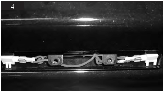
4.6 Fit ceramic block and fit thermometer
