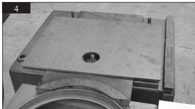
1.4 Set top conducting plate in position.
