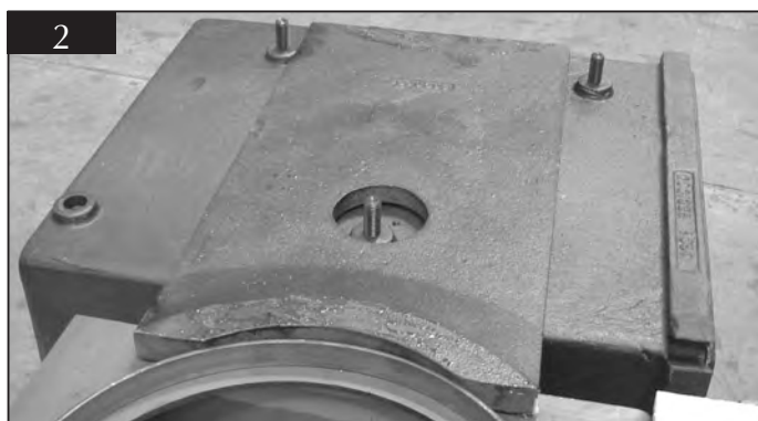
1.2 Set conducting plate (part C600582) in place on lower oven.
