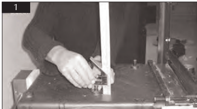
1.1 Set Top Oven conducting plate studs to 30 mm high.
