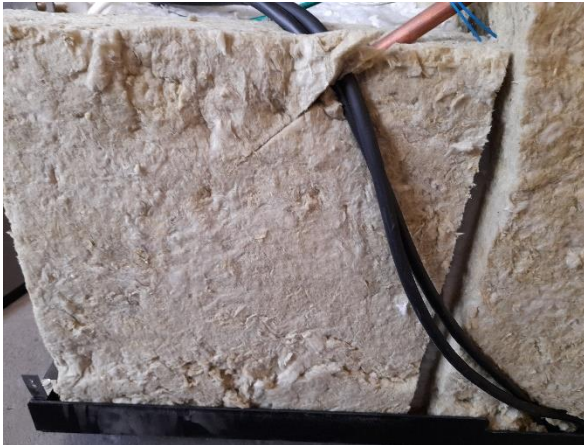
Remove the insulation to gain access to warming oven element
