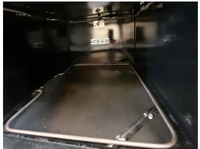
Fig13.Lower oven base element.
