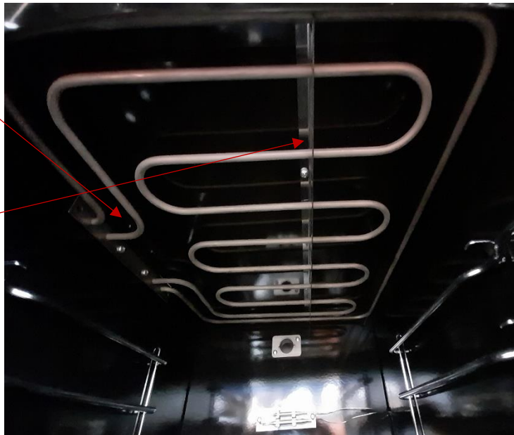
Grill element securing screws
