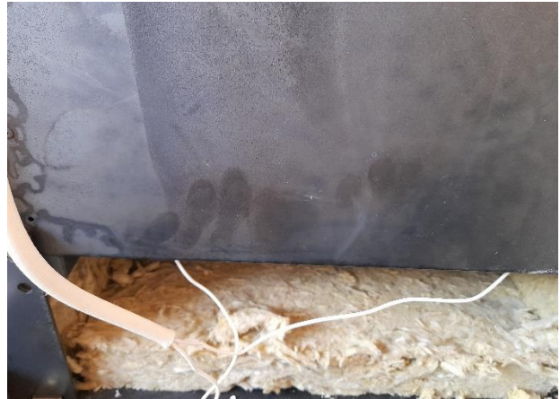
Remove the insulation to gain access to warming oven element
