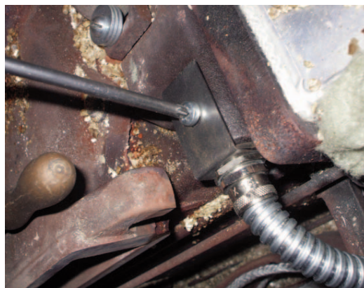
FIG. 4 FIT LOCATION BRACKET TO TOP OVEN
