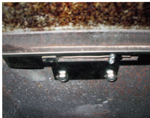
FIG. 8 ATTACH PHIAL PLATE (AS SHOWN)
