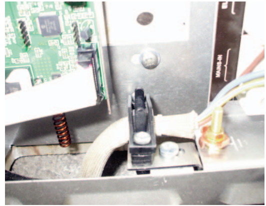
FIG. 2 FIX CABLE CLAMP TO CONTROLS PANEL
