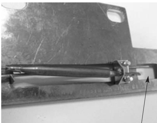
FIG. 7 POSITION ELEMENT AND OVERHEAT SENSOR
