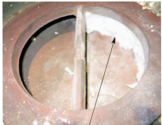
FIG. 8 FIT PAD BELOW SIMMER PLATE
