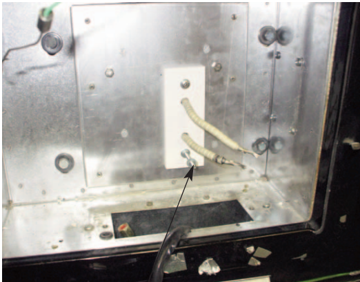
FIG. 5 M5 STUD FITTED TO BURNER DOOR
