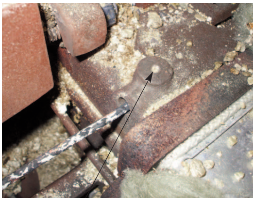
FIG. 1 DRILL AND TAP HOLE (M6)
