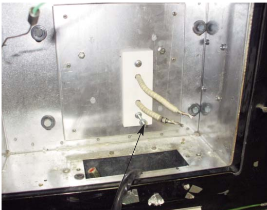
FIG. 5 M5 STUD FITTED TO BURNER DOOR
