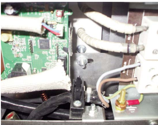
FIG. 5 M5 STUD FITTED TO BURNER DOOR
