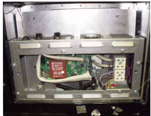
FIG. 6 FIXINGS FOR CONTROL BACK COVER (M5) NUTS, WASHERS PLUS 2 SCREWS
