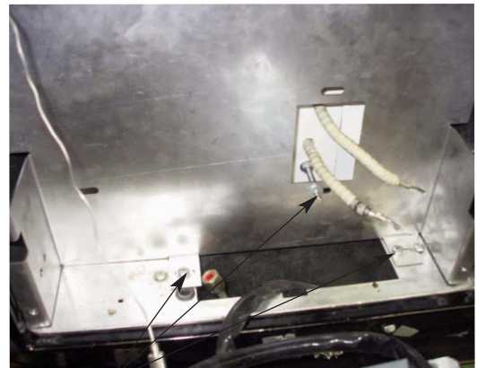
FIG. 6 FIXINGS FOR CONTROL BACK COVER (M5) NUTS, WASHERS PLUS 2 SCREWS
