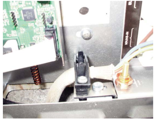
FIG. 2 FIX CABLE CLAMP TO CONTROLS PANEL
