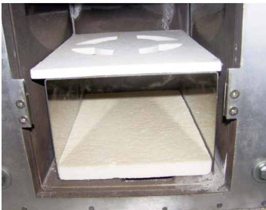
FIG. 5 PLATFORM AND PADS INTO ASHPIT
