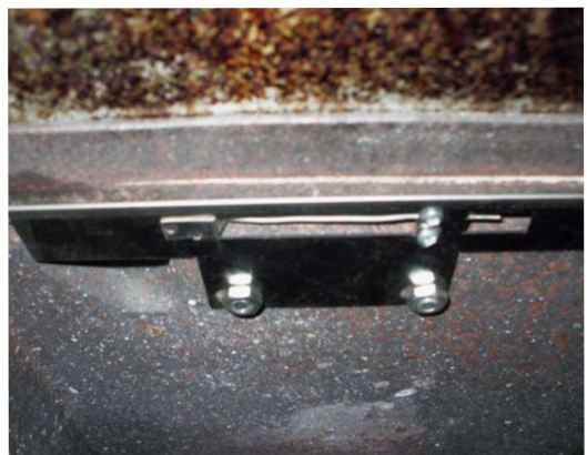
FIG. 8 ATTACH PHIAL PLATE (AS SHOWN)
