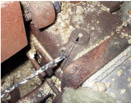
FIG. 1 DRILL AND TAP HOLE (M6)
