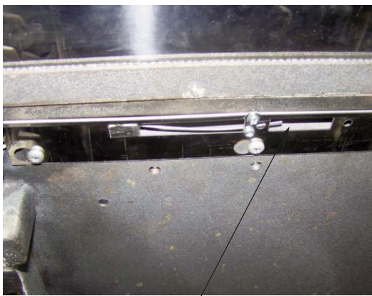
FIG. 2A POSITION THEROCOUPLE (10mm SPACING)
