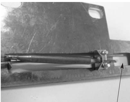
FIG. 7 POSITION ELEMENT AND OVERHEAT SENSOR 10mm SPACING
